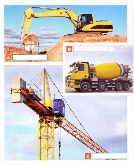
A tower crane is used to build tall buildings. Its short arm carries a counterweight of concrete blocks and its long arm carries lifting gear. The operator can sit in a cabin at the top of the tower just below the horizontal boom or control the crane by radio remote control from the ground. The lifting hook is controlled by a system of sheaves.
