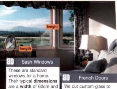
a height of 90 cm. The bottom sash opens. The top sash is fixed.
