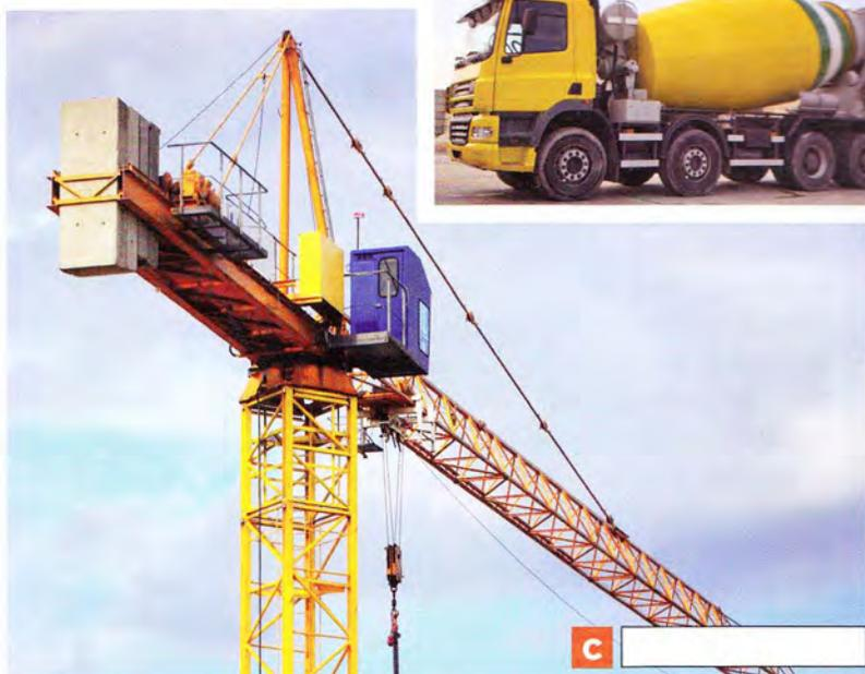
A **tower crane** is used to build tall buildings. Its short arm carries a counterweight of concrete blocks and its long arm carries lifting gear. The operator can sit in a cabin at the top of the tower just below the horizontal boom or control the crane by radio remote control from the ground. The lifting hook is controlled by a system of sheaves.
